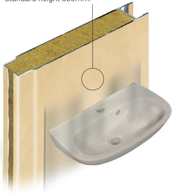
Standard reinforcement for other wall hung equipment.
